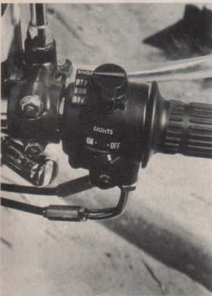
At least one Japanese motorcycle manufacturer still allows the motorcyclist to decide if the headlight is to be on at all times.
